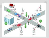
Topologically volatile network made up of AVs supporting the DSRC protocol.
